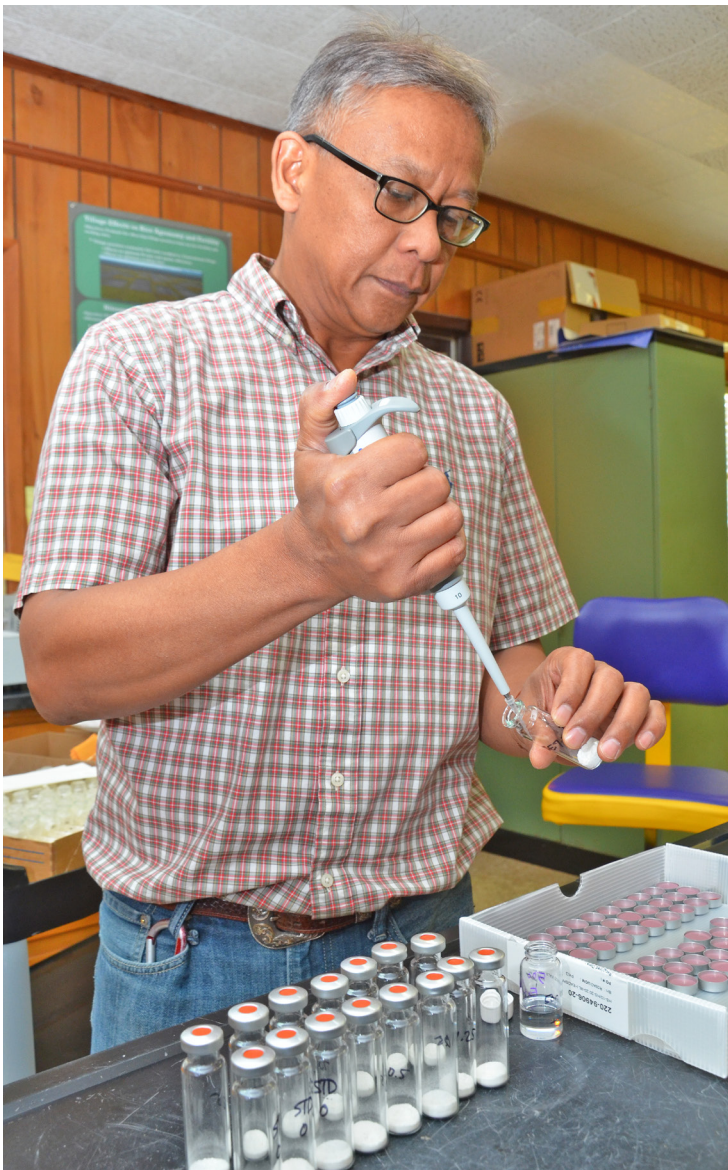
AgCenter rice agronomist Manoch Kongchum inserts a sample of a Jazzman rice line to be analyzed by a gas chromatograph for the proper aroma trait. Kongchum tested 15 lines of Jazzman with the Clearfield trait, and one will be selected to be grown as foundation seed at the H. Rouse Caffey Rice Research Station in 2017.
